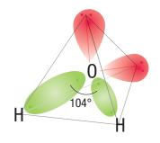
Non-bonding pairs take up more space than bonding pairs, so the angle between the bonds is 104° instead of 109°, which would be the angle at the center of a tetrahedron.
