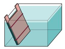
4) If at this point you hook a digital multimeter to the terminals (tabs), you will notice that the battery is producing a current of a few millivolts. This is due to impurities in the metal that are not uniformly distributed across the two sheets. This occurs even if you cut them from a single sheet of copper.
