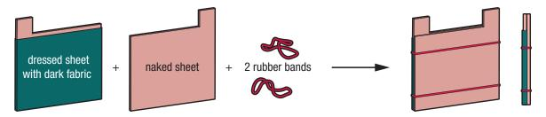
The naked sheet will be the one exposed to the light, while the other will be kept in the dark by the fabric around it. Before continuing, make sure that the two sheets are not touching anywhere.
